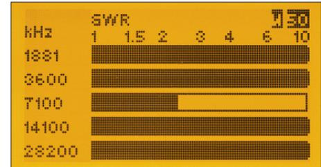
Fig. 23: Simultaneous SWR measurements on 5 programmable frequencies
