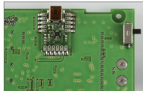
**Fig. 4: USB interface board correctly positioned**
