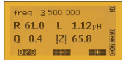
Fig. 33: In the mode LCR meter, the FA-VA5 displays the measured values in a large and clear representation.
