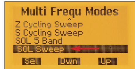
**Fig. 14:** SOL compensation for the actual Frequencies for a multi-frequency measurement
