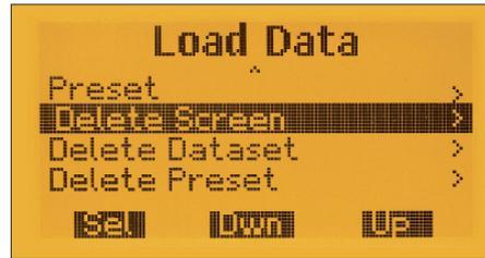
Fig. 36: Menu items for deleting stored Screens, Datasets and Measurement Presets.
